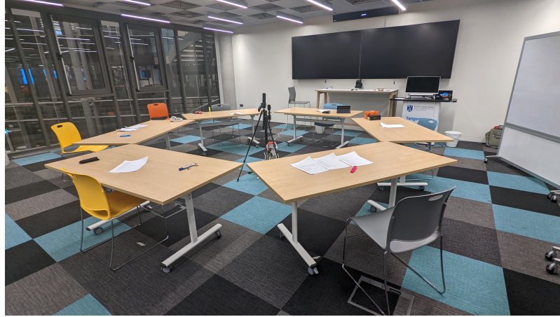
Fig. 1. Side view of the set used for recording stimuli. Omnidirectional camera and ambisonic microphones can be seen in the centre.
